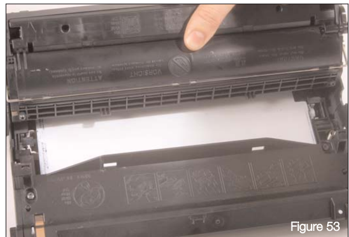
Lift the OPC Assembly from the Drum Unit.
